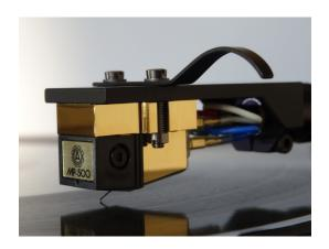
Output Voltage 3,0 mV (5 cm/sec) Frequency characteristics 20-25.000 Hz Channel Separation 27 dB (1 KHz) Channel balance 1.0 dB or less Load resistance 47 KΩ Cantilever Boron Stylus tip shape/radius Line contact Stylus tip material naked diamond Stylus pressure 1,3 - 1,8 gCartridge weight 8,0 g
