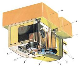
for the MP-100 and MP-110 which have a light weight bonded diamond tip), which is only one third of the mass of conventional diamond tips. It is manufactured by super fine particle grinding, based on extended stylus technology.
