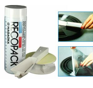
This is a cleaning system for very dirty records. A special syrup is distributed on the record using the supplied dispenser. A removal tag is placed on the edge of the record, halfway, in the still fluid syrup. Then the syrup is allowed to dry into a film during 24 hours. Once the film is dry you can remove it carefully by lifting the tab. All parts that do not belong to the record are now trapped in the film, even residue from previous use of for instance Lenco clean fluid.
